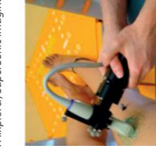
Figure 1 : (a) Stiffness assessment using an innovative, freehand, experimental setup composed of a force sensor mounted in series with an ultrasound probe (b) Experimental and simulation curves of the force-displacement response for the seven subjects
